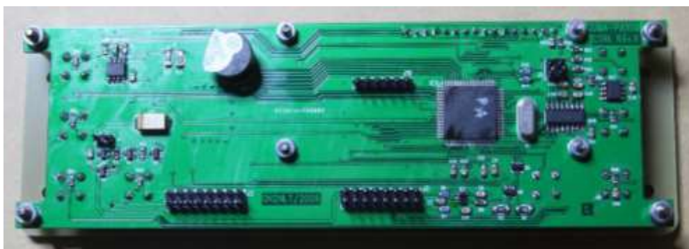
Figure 15 Digital Control Board – Rear View with all components in place.
