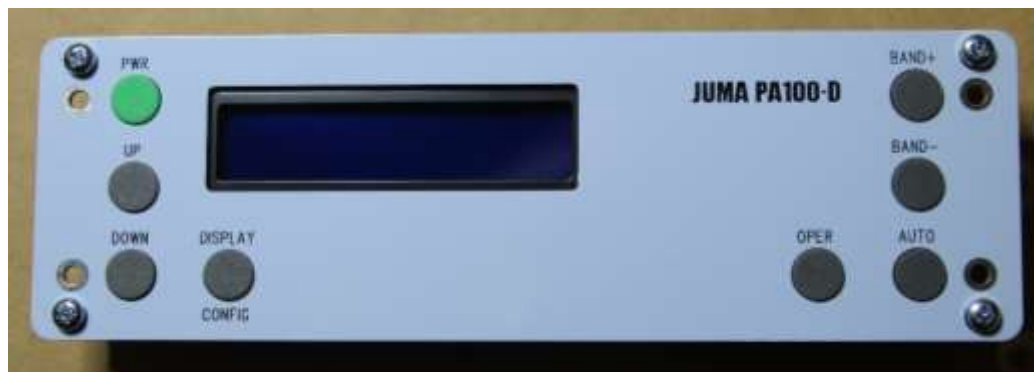
Figure 17 Digital Control Board – Front View with pushbuttons in place and front panel fitted.
