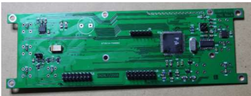
Figure 11 Digital Control Board – Bottom View with PIC and Crystal Installed.
