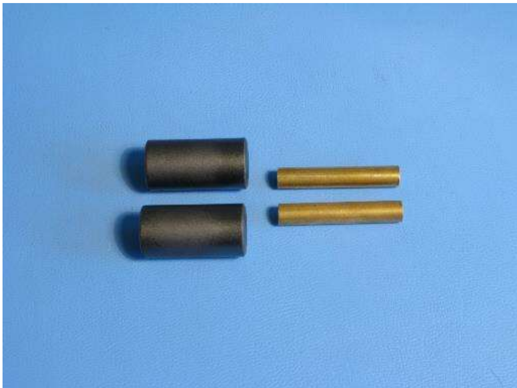
Figure 18 Transformer T2 ferrites and the brass tubes. Smooth the inside edges of the tubes if needed.
