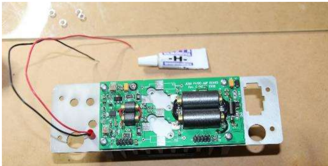
Figure 35 VK4GRM - PCB fixed in place with the rear plate and the heatsink
