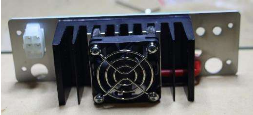
Figure 47 VK4GRM - Completed amplifier module – Rear View.
