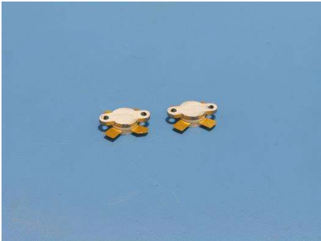
Figure 37 Apply thermal grease to the final transistors
