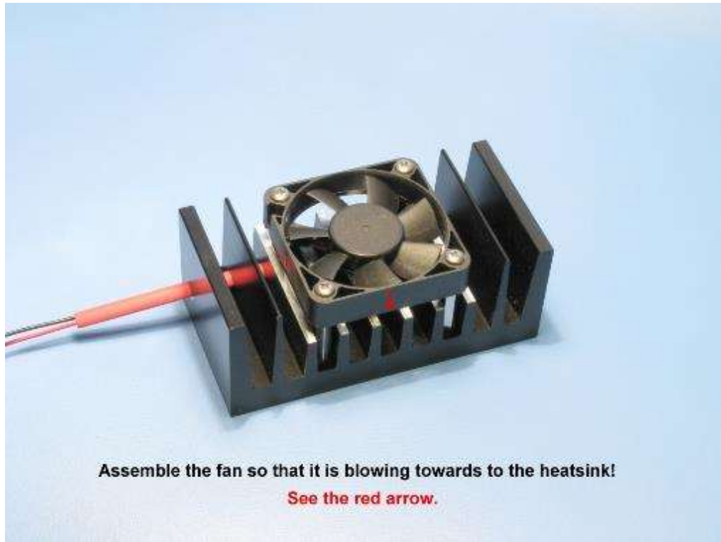
Figure 26 Install the fan with the finger shield to the heatsink. (Finger shield missing in this picture).
