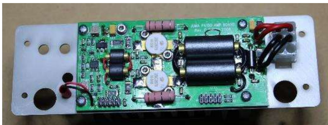
Figure 46 VK4GRM - Completed amplifier module.
