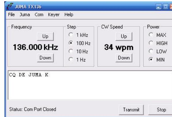
The JUMA TX136-500 software can use to perform QSO with the CW, QRSS, DFCW, JASON, WSQ and JT9 modes.
